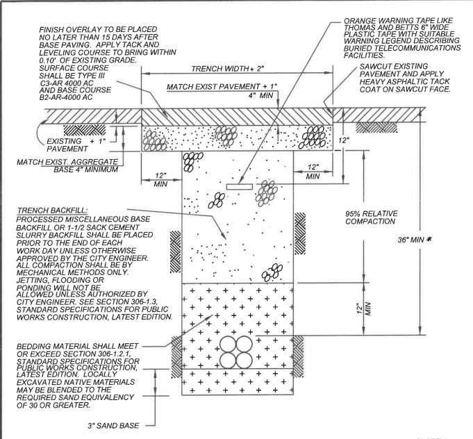
\* 36" MIN FOR TRUNK AND DISTRIBUTION CONDUIT SYSTEM AND 18" MIN FOR SERVICE LATERAL CONDUIT SYSTEM.
